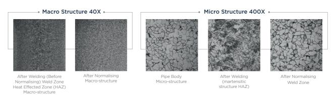
After heat treatment, the pipe body and welding line microstructure have the same homogeneous structure and hardness.
